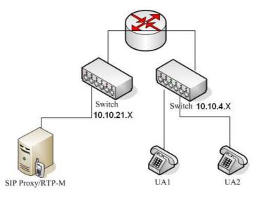
Figure 16: SIP Proxy Server and UAs on different Subnets
