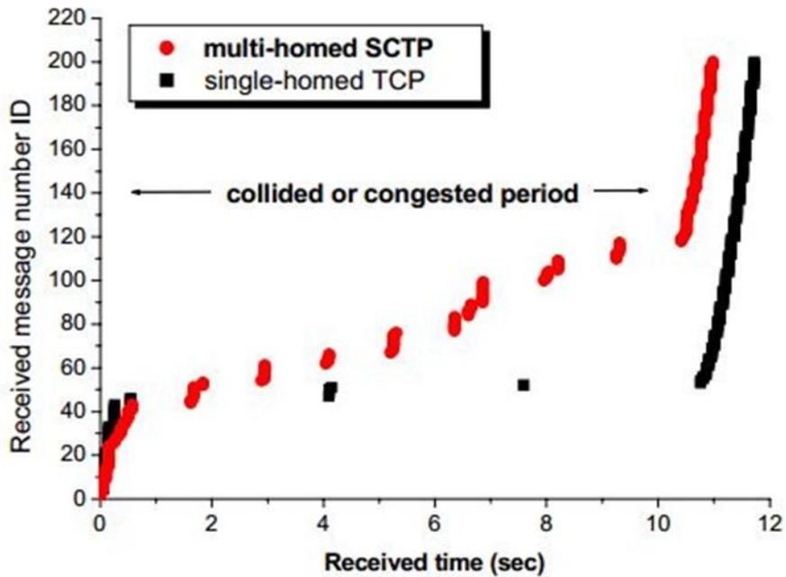
**Figure 4 Alternate retransmission of SCTP vs TCP**
