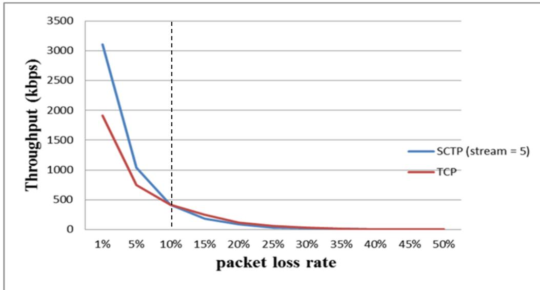
**Figure 10 The throughput of SCTP and TCP (multi-streaming)**
