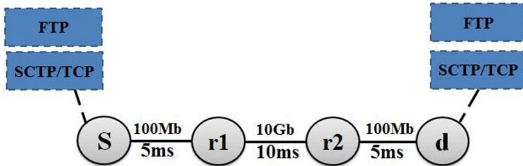
**Figure 9 Network topology of the multi-streaming test scenario**
