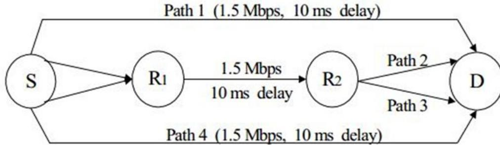
**Figure 5 Simulation networks topology**
