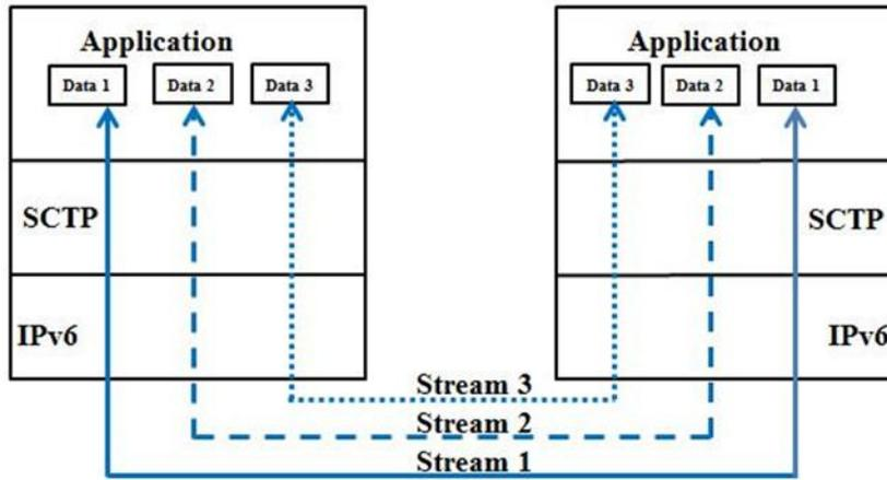
**Figure 8 Sctp multi-streaming mechanism**
