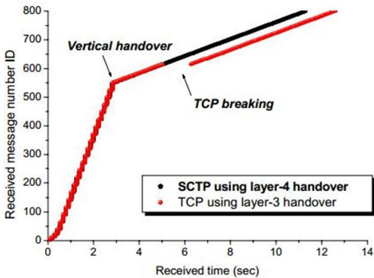
**Figure 2 Vertical handover in layer4 vs layer3**
