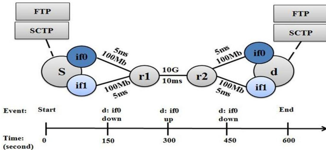
Figure 11 Network topology of the multi-homing test scenario
